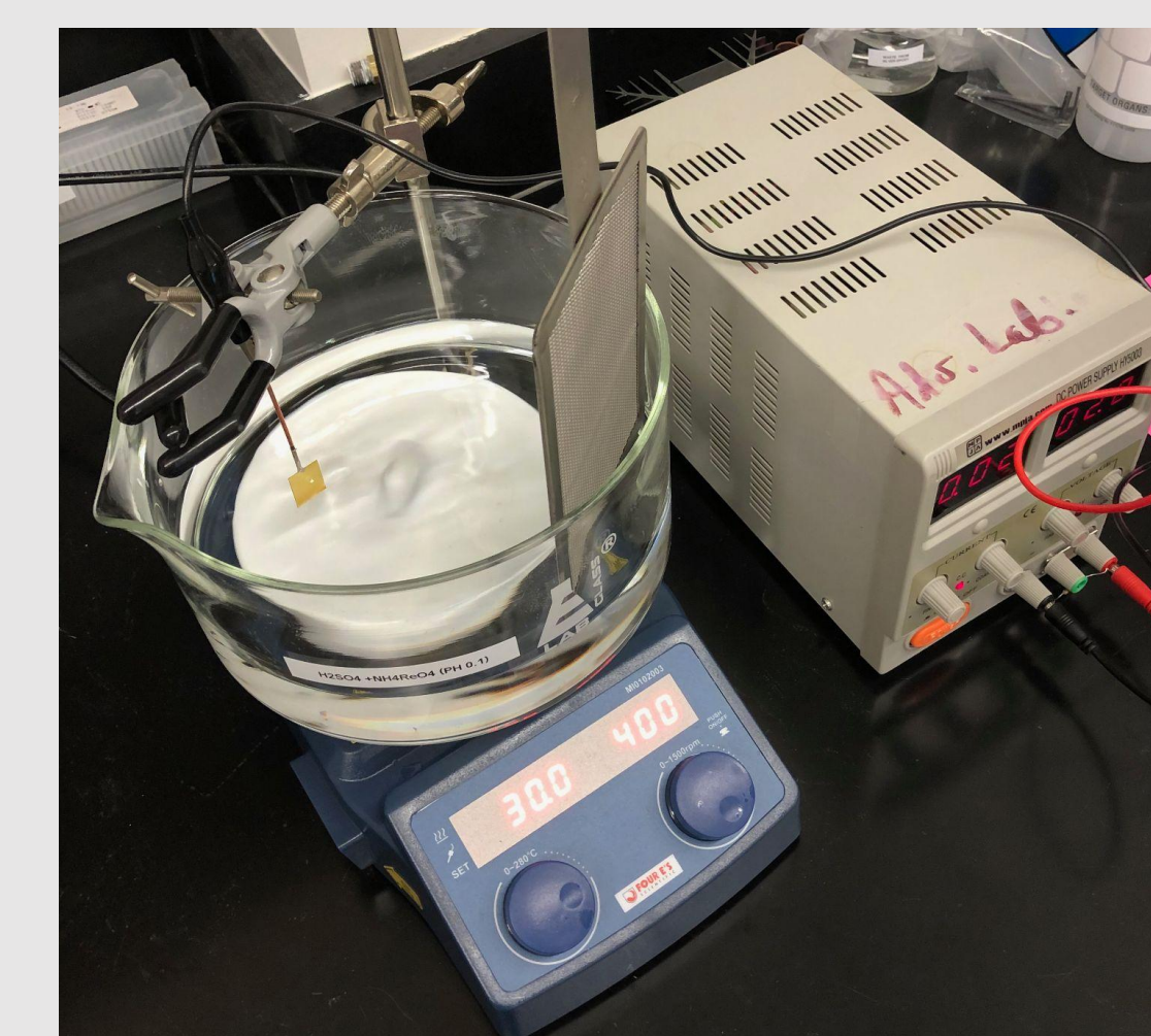
The experimental setup. The substrate hung from the black wire and was dipped in the solution. The platinum anode was attached to the red wire.
